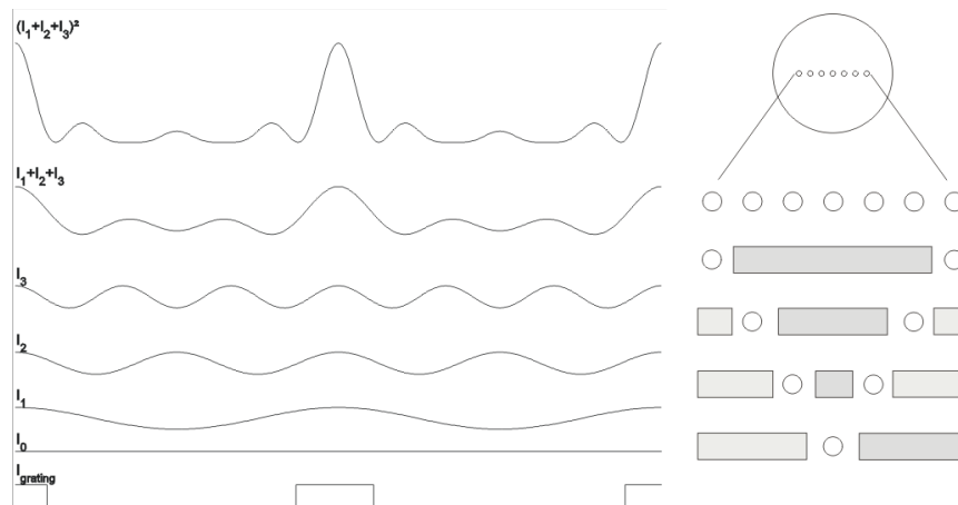
Figure 2 Plot showing the image of a grating when blocking different diffraction orders (as shown to the left). I_{\text{grating}} shows what the intensity image of the grating should look like.
