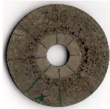
corroded Mg plate
