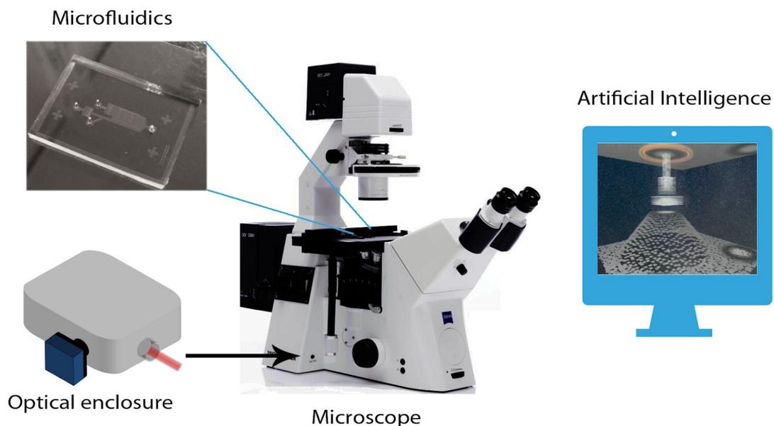
*Fig. 1 | Lucero's single-cell micromanipulation platform. Lucero's solution is based on an enclosure with the necessary components to provide Holographic Optical Tweezers (HOT module) to any inverted microscope through the camera port. In combination with application-specific microfluidic chips and a user-friendly software based on Artificial Intelligence (AI).*
