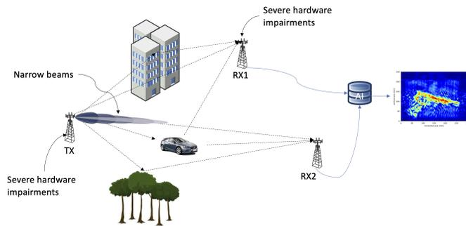
Fig. 1. Considered multi-static setup where the signals at the different receivers are processed to create a 3D image of the environment. The goal of this project is to develop the AI unit, based on models of the propagation, signals, and hardware limitations.
