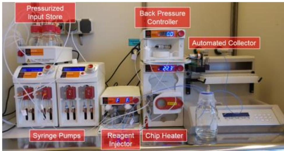
Fig. 1 Asia flow system (installed in lab 8120)
