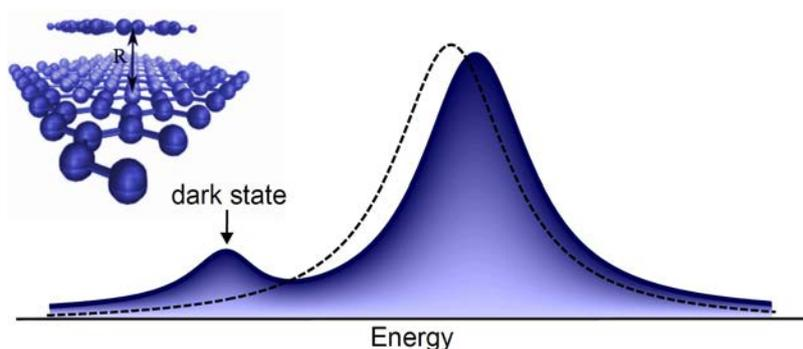
**Fig.1.** Excitonic absorption spectrum of pristine (dashed) and molecule-functionalized (blue filled) tungsten disulphide ( $\text{WS}_2$ ). The presence of high-dipole molecules activates dark excitons resulting in a new resonance at the lower energy side of the bright exciton.
