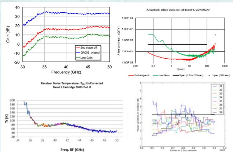
Fig. 2: Receiver noise, system stability, power variation in 2GHz window after switching off LNA 2<sup>nd</sup> stage.
