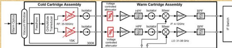
Fig. 3: Proposed system block diagram for solar flare observation.
