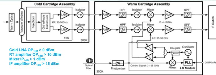
Fig. 1: Block diagram of ALMA Band 1 receiver front-end.
