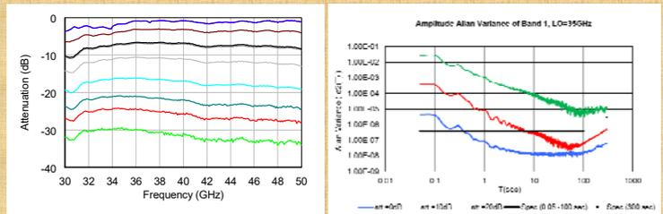
Fig. 4: Dynamic range of commercial VCA and system stability with VCA.
