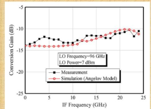
Fig. 2: Mixer operating at Band 2+3 frequency: (left) chip photo. The chip area is 1mm x 1mm; (right) simulated versus measured conversion gain of the mixer.
