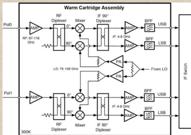
To cover extremely wide RF bandwidth, 2SB down-converting scheme is proposed to obtain reasonable LO fractional bandwidth (75-108 GHz, 36%) with 4-8 GHz IF frequency band. IF amplifier is optional to provide flexible IF output power control.
