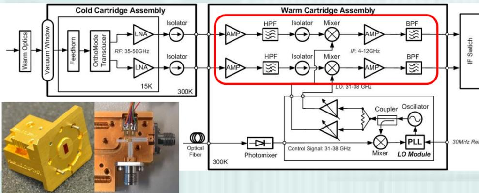
Fig. 1: Block diagram of ALMA Band 1 receiver front-end. Down-converter is circled in red. (Lower-left) Photo of the in-house designed MMIC mixer module.
