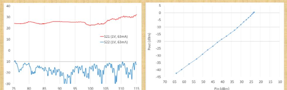
Fig. 3: RT Amplifier operating at Band 2+3 frequency: (upper) chip photo. The chip area is 1.25mm x 0.66mm; (lower left) Measured gain and output return loss of the amplifier and (lower right) Measured input power versus output power at 100 GHz.  $P_{1dB} > 0$  dBm.
