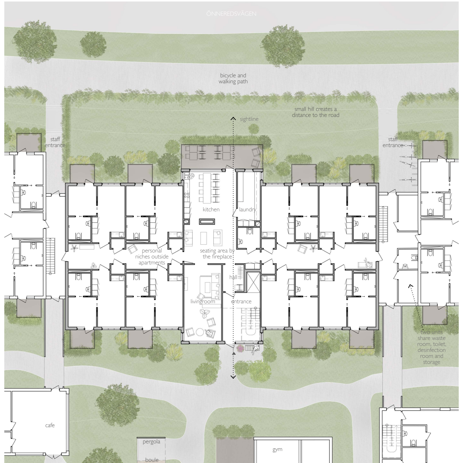
8 apartments unit, groundfloor 1:200 0 1 5 10 m N
