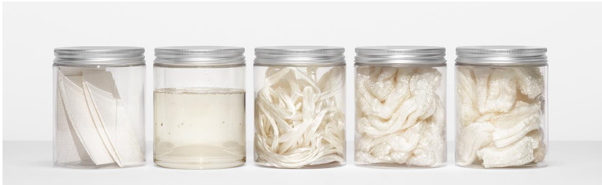
Figure 3: Five jars containing samples from various process steps in the TreeToTextile process: sheets of dissolving pulp, spin-dope (dissolved cellulose), filaments, crimped fibers, cut staple fibers.
