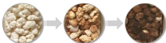
Figure 4: Color change of the cellulose-silica adsorbents during exposure to VOCs
