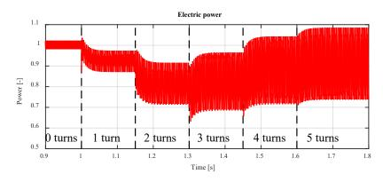
Figure 2 The output power of the converter driven model during generator mode.
