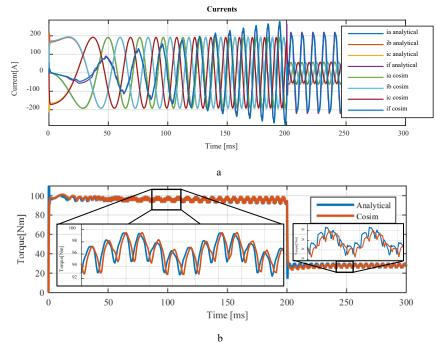
Figure 1 Currents and torque from analytical model and the co-simulation which includes the FEM model during ideal converter operation. The torque reference is stepwise reduced from 100 Nm to 30 at 200 ms.
