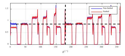
Figure 3 Normalized normal component of the air-gap flux density for one time instance during generator operation for faulted and non-faulted machine model
