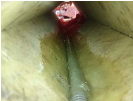
Figure 22 Wooden box with an imbedded tube where an electrical cable can be placed.
