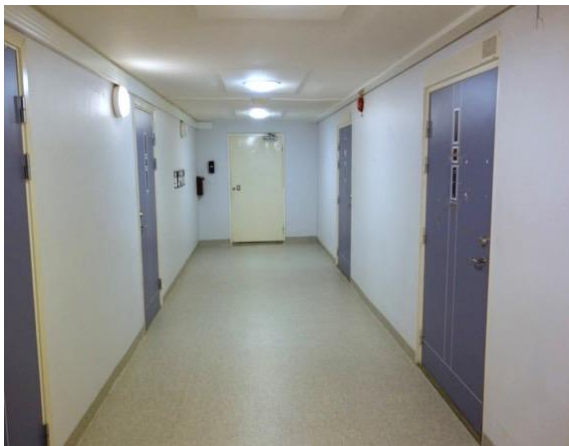
Figure 9. Most SiS living units visited by the author and other Chalmers University researchers had prominent corridors. Some unit floor plans were dominated by long corridors or hallways. Studies on correctional facilities and other types of locked treatment settings have reported that corridor-dominated floor layouts hinder observation and are linked with increased rates of aggressive behavior and rule violations (Sections 7.1 & 7.2). The design model proposed in the report does not consider corridors to be rooms, and excludes them in calculating social density. Fire codes often prevent placement of seating and other furniture in corridors of locked treatment facilities. (Photo by R. Ulrich)
