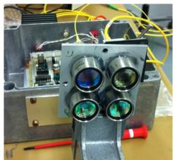
Figure 3: LIDAR sensor for ice detection
