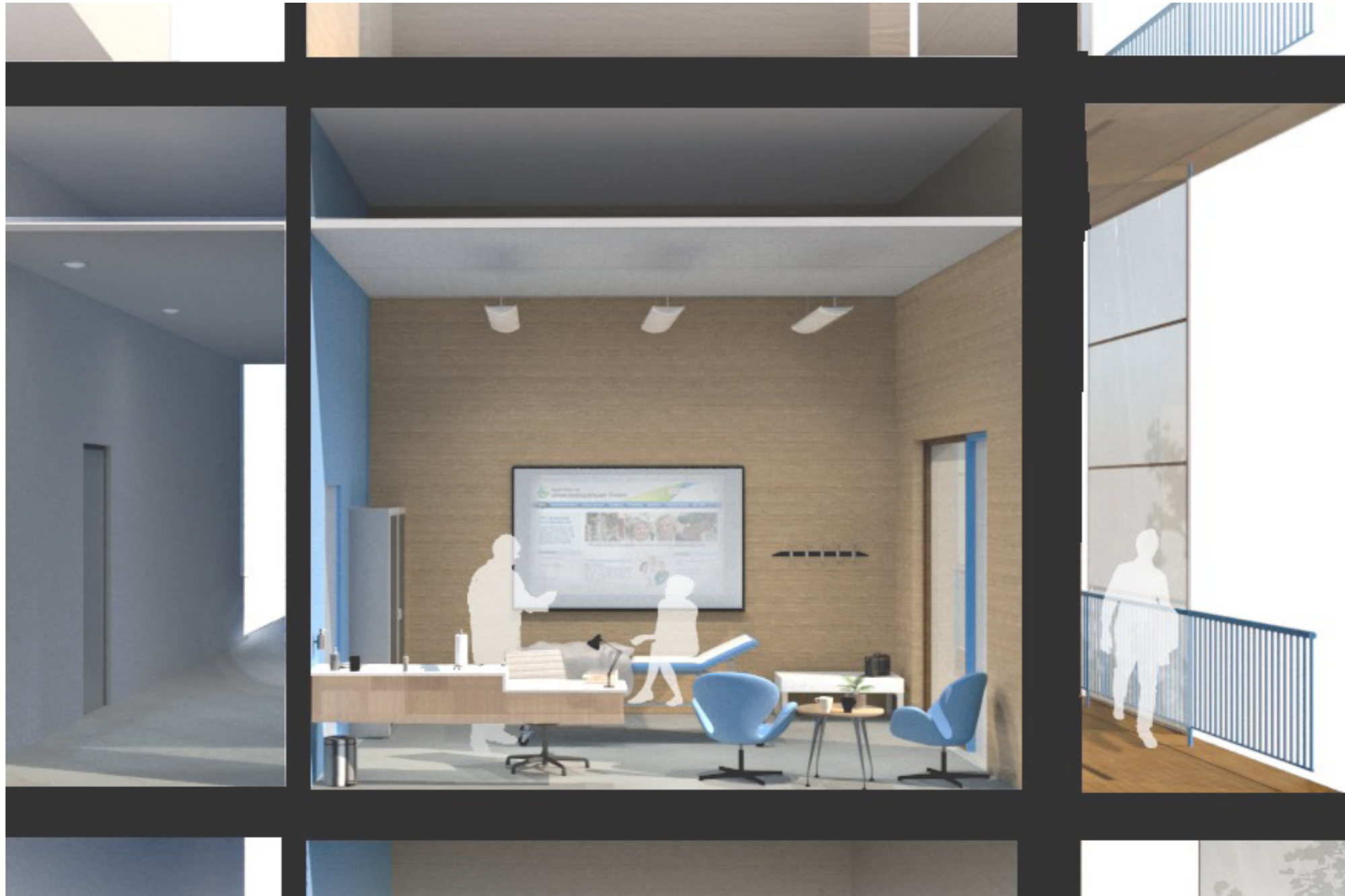
Section through an examination room, where the patient enters from the open gallery and staff from the corridor.
