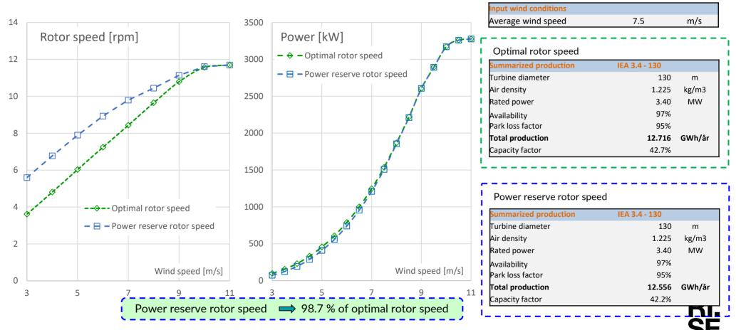
Comparison of AEP between operation at optimal rotor speed vs. power reserve speed
