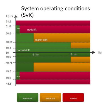
"The main objective for FCR-D upwards is to secure frequency stability, i.e. that the power system **frequency does not decrease below 49.0 Hz**. The largest reference incident in the Nordic power system is a trip of the nuclear power plant Oskarshamn 3 at 1450 MW. "
