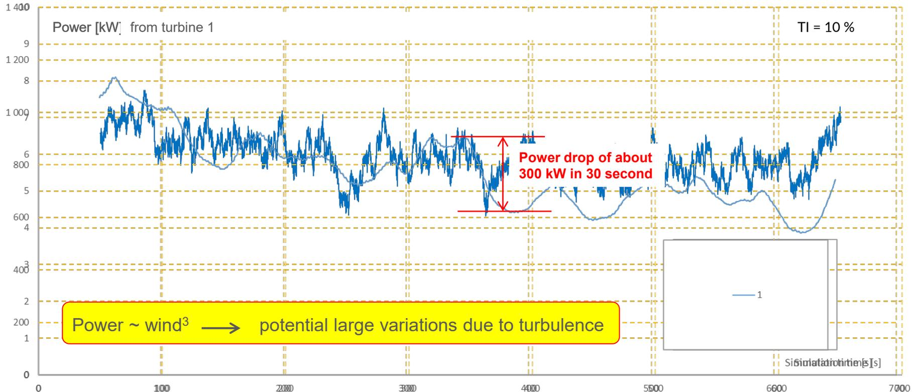
It is not possible to run a turbine at constant power for longer times in low wind speeds
