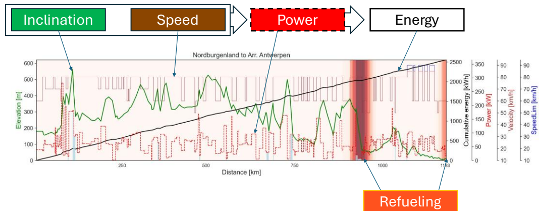
Figure 21: One simulated route. The x-axis represents distance driven along the route. Elevation (green) and velocity (brown) impacts power (red), which results in a total cumulative fuel demand (black). Where the power is accompanied by a light blue bar, the power needed ( P_{link} ) is negative and is utilized for regenerative braking, which in turn decreases the cumulative fuel demand. Refueling demand allocated to nodes along the route is depicted with vertical shaded areas. Speed limit (blue) is included to specify where the truck runs slower than the speed limit
