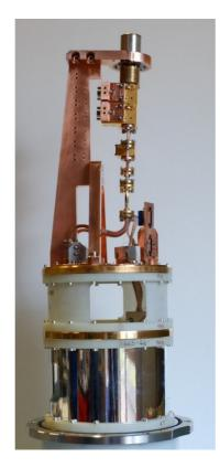
*Figure 7. Early ALMA Band 2 (+3) cold cartridge prototype*
