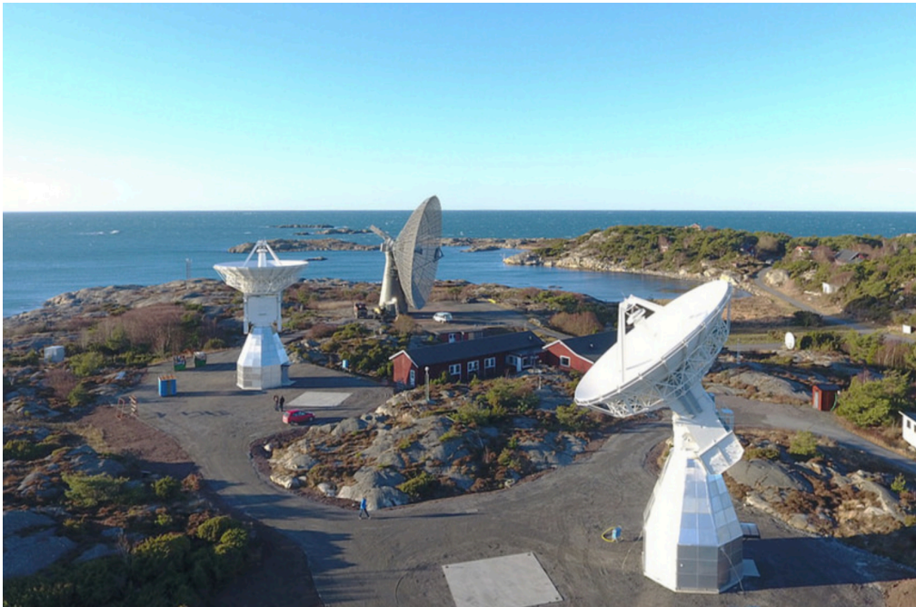
Fig 4. In foreground is the new Onsala Twin Telescope for geodetic VLBI formed from two 13 m diameter dishes. Behind these is the 25 m diameter telescope used for astronomical VLBI.
