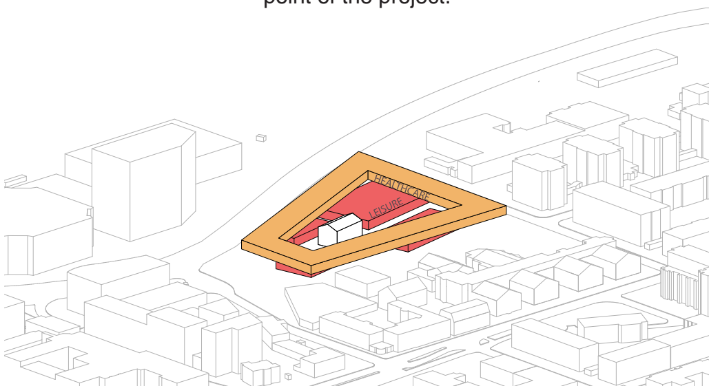
Fig. 4 The second floor is added and designated to become the patient floor; its geometry takes into account the built environment.
