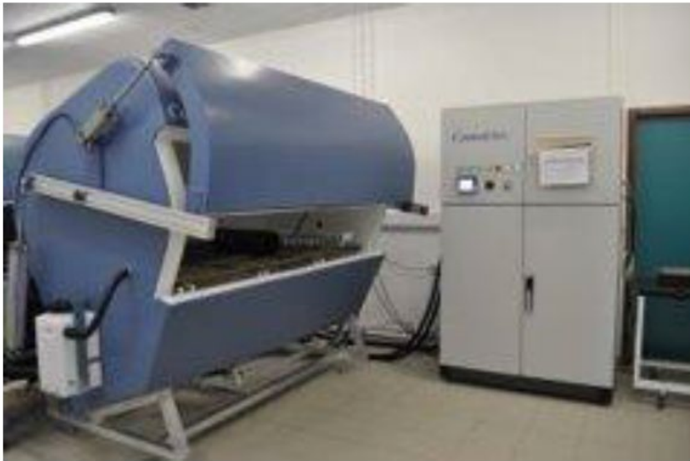
Accelerated corrosion test cabinet (salt spray) at RISE (Kista).
