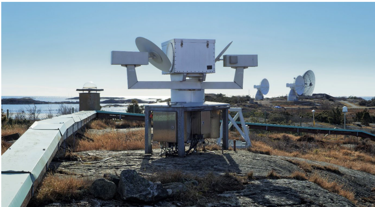
Figure 1.2. The water vapour radiometer Konrad and othe geoscience instruments in Onsala, with the twin telescopes and the 25 m telescope in the background. Credit: Magnus Thomasson
