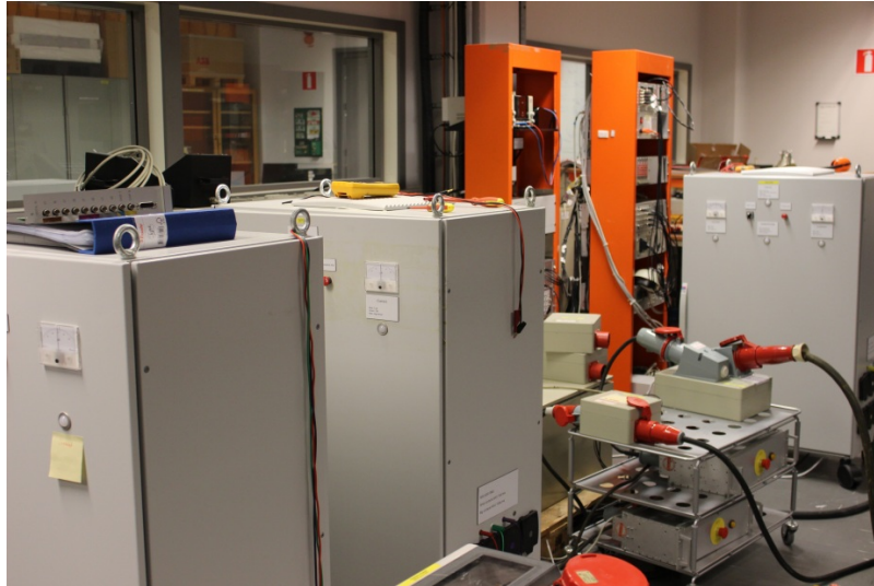
Figure 8: Laboratory setup: modelling of the back-to-back VSC and wind turbine.
