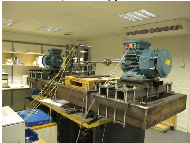
Figure 9: The test rig of high-speed subsystem of drive train of a wind turbine
