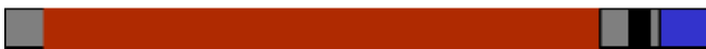
Figure 22: Model of the plate with ice. From left gray is glass fibre laminate, red is core material, gray glass fibre, black carbon fibre, gray gelcoated surface and blue ice.
