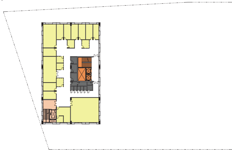
■ PSYCHIATRY (STAFF) ■ EMERGENCY CORE ■ CIRCULATION CORE ■ STAFF-GOODS CORE ■ SUPPORT-TECHNICAL ■ GOODS SCHEMATIC FLOORPLAN NO SCALE
