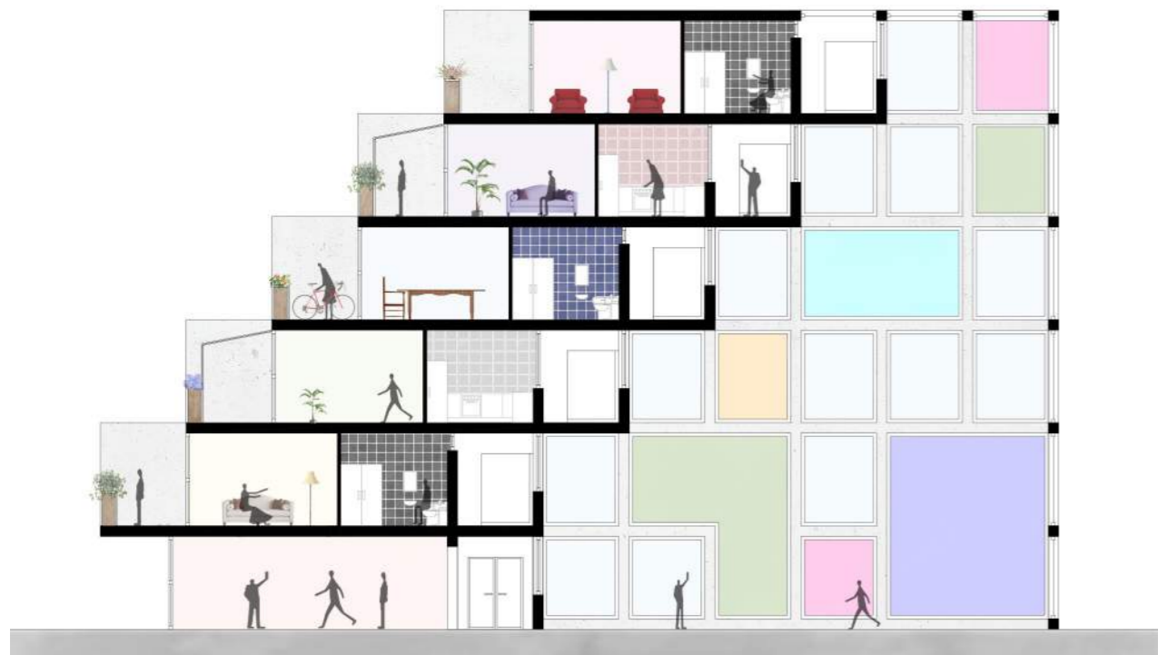
SECTION THROUGH APARTMENTS (1:200)
