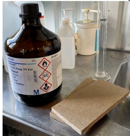
Fibre board (200x95x10mm) soaked with 1 dl methanol
