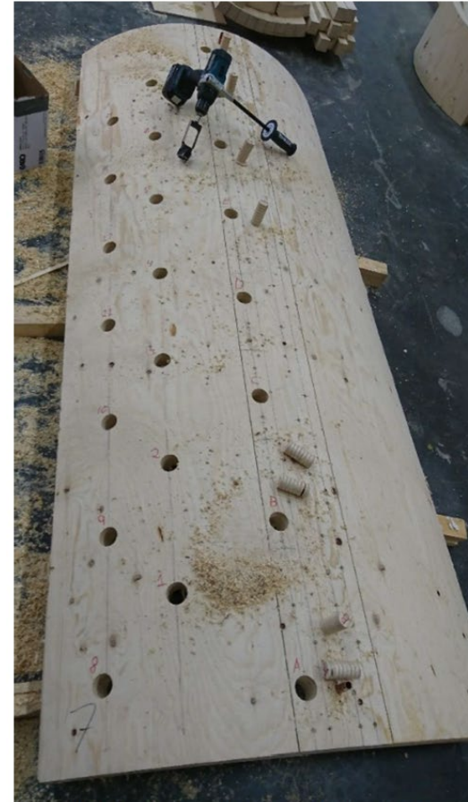
Figure 2 Making test specimens from the laminated module
