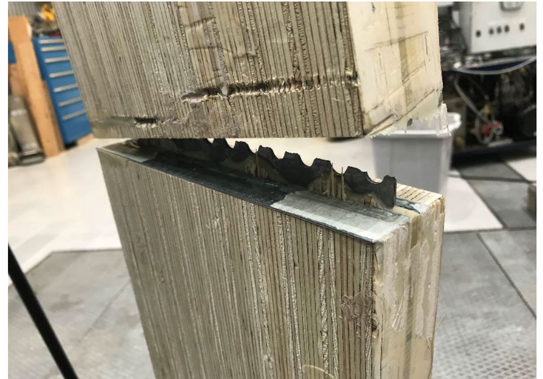
Picture of the tested samples with cyclic loading Test sample nr. 7
