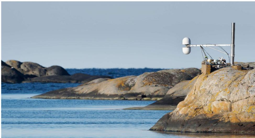
*Figure 1.2. The GNSS-based tide gauge in Onsala. Credit: Magnus Thomasson*
