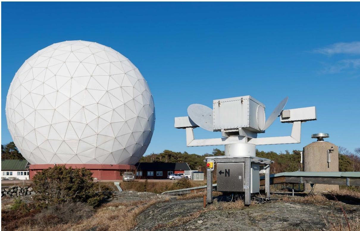
**Figure 1.3.** The water vapour radiometer Konrad, with the radome enclosing the 20 m telescope in the background. Credit: Magnus Thomasson
