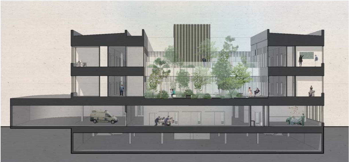
SECTION A-A Ambulance garage and resting garden
