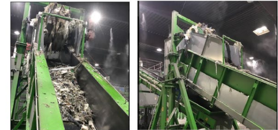
D. Secondary shredder and homogenisation with RDF
