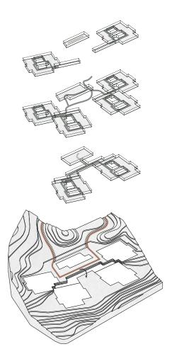
Within the facility a good flow of movement for the residents and staff needs to be ensured and is created through connecting all the building parts through indoor and outdoor pathways.
