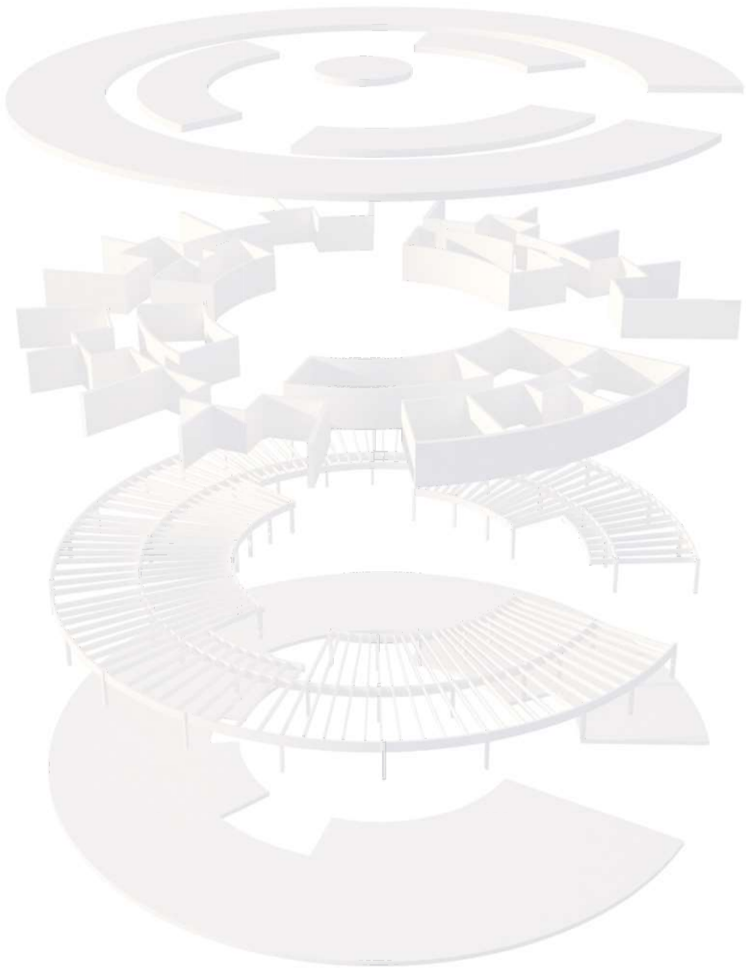
wooden pillars and beams
