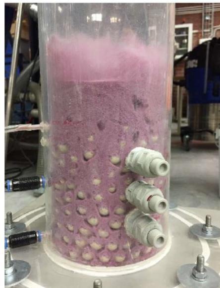
The arrangement has a number of potential advantages, notably improved gas-solid mass transfer due to strict limitations on bubble growth.
