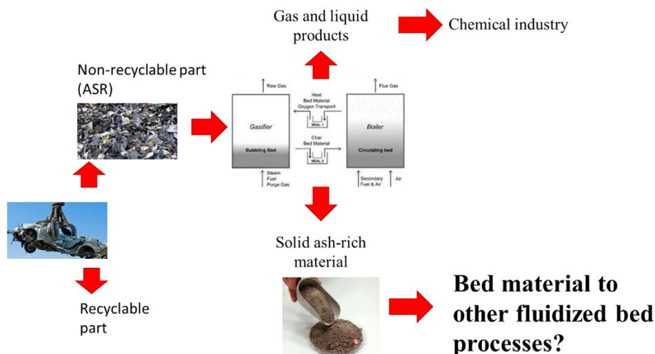
Our suggestion is that this material can be used as bed material for other fluidized bed processes, e.g. as a catalyst, an oxygen carrier or an inert bed material. Your
