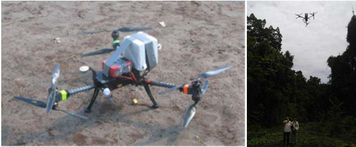
Drone with attached MultiGas instrument, tested at Bagana volcano, Papua New Guinea, in September 2016.
