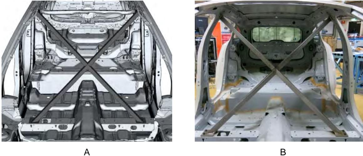
Figure 7: Beam cross to increase torsional stiffness – Simulation (A) and Test (B)
