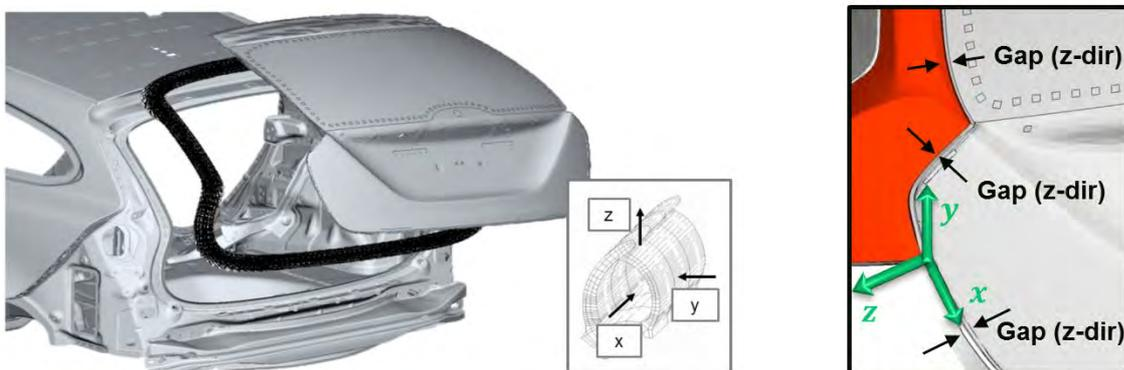
Figure 6: Sealing represented by spring elements – local gap direction
