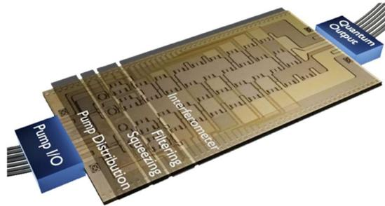
*Photonic Chip realizing a Continuous-Variable quantum computer on the cloud, courtesy of Xanadu*
