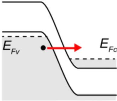
Figure 2. Band diagram of a reverse biased tunnel junction.
