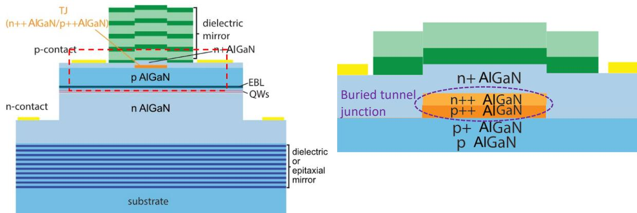
Figure 1. (left) Schematic view of a TJ VCSEL and (right) a zoomed-in view of the TJ.
