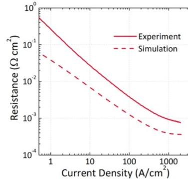
Figure 3. Simulated and experimentally measured tunnel junction (p-AlGaIn/InGaIn/n-AlGaIn) resistance [1].
