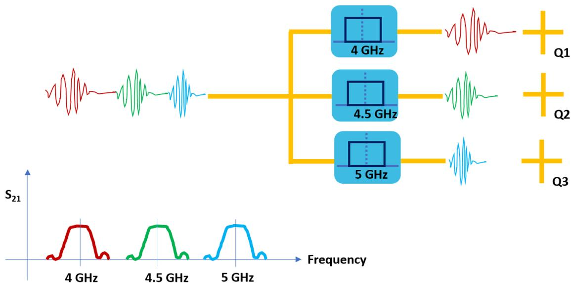
A bank of band-pass filters separates and forwards each pulse to its corresponding qubit. The number of XY or drive cables is reduced by a factor of 3 in this simplified example.
