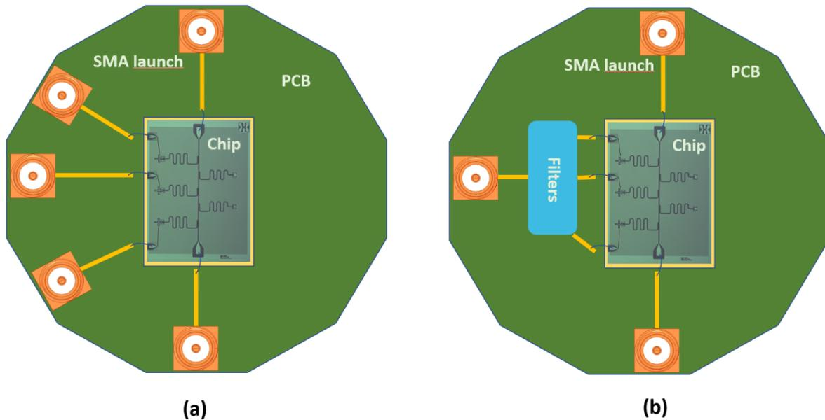
Design (a) shows a simple example where each qubit has its own XY-line, therefore three SMAs on the left side of the PCB and three cables are required. In design (b), a triplexer filter reduces the number of SMA/cables to three. The incoming pulse is directed to its corresponding qubit depending on the frequency.
