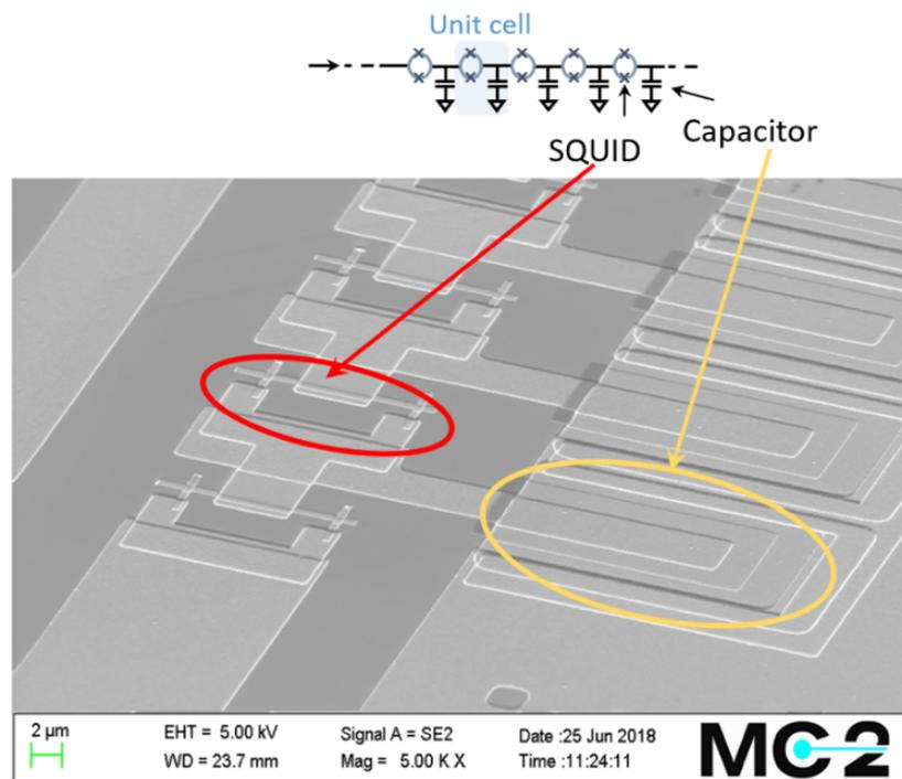
A travelling wave parametric amplifier (TWPA) made of approx. 500-unit cells. Each unit cell has one SQUID (composed of two JJs in parallel) and a parallel capacitor to ground.
