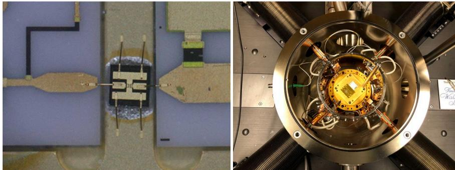
The InP transistors in LNA and the cryogenic measurement set-up
