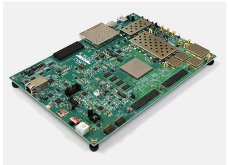
*The Xilinx Zynq® UltraScale+™ Radio Frequency System-on-Chip (RFSoc) that you will use in this thesis.*
