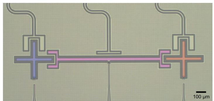
*Elementary quantum processor consisting of two superconducting qubits (blue, red) connected by a coupling element (purple). Micrograph courtesy of A. Bengtsson.*
