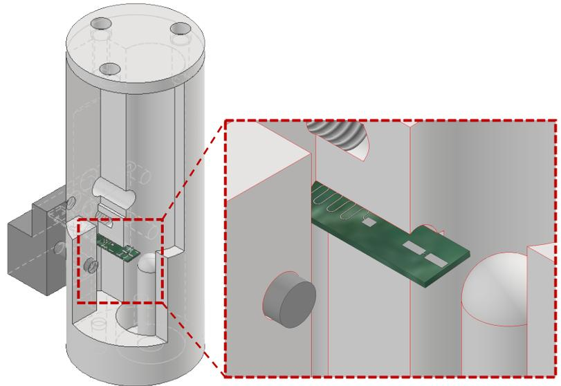
3D rendering of a high-Q coaxial microwave cavity used in our experiments [3]. Close-up: a silicon chip with a superconducting qubit and a readout resonator is inserted into the cavity to prepare, manipulate, and read out nonclassical states in the cavity.
