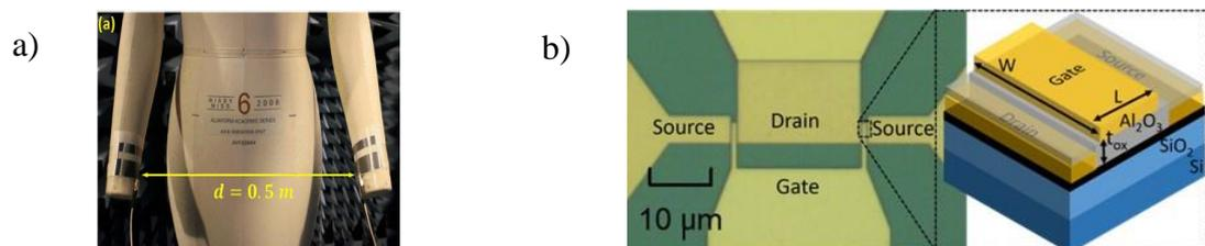
Fig. 1: a) Wearable graphene THz antennas on mannequin (X. Huang, T. Leng, M. Zhu, et al. Scientific Reports, 5:18298, 2015), b) microphoto and schematic of a fabricated GFET on Si substrate with two gate fingers (M. Bonmann, A. Vorobiev, M. A. Andersson, and J. Stake, Appl. Phys. Lett. 111, 233505, 2017).
