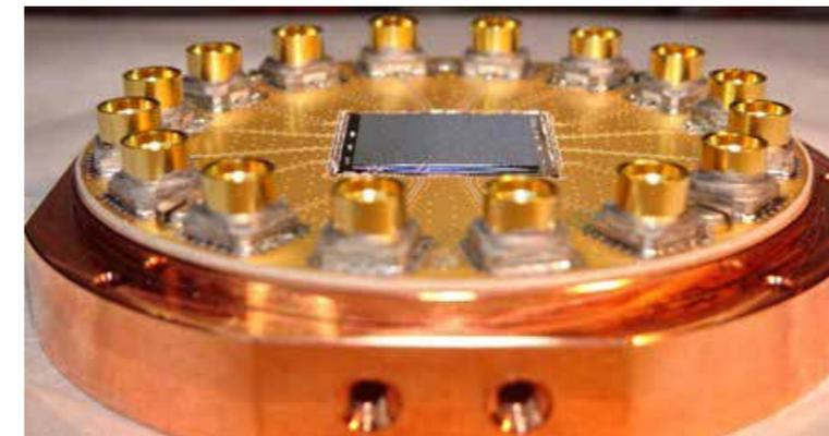
Quantum computer chip mounted in a sample holder before measurement
