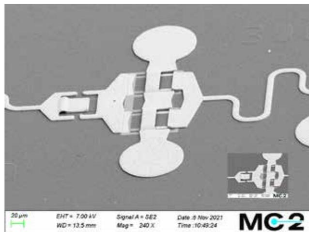
SEM-images of a simple GaN-based MMIC and a close-up of the transistor fabricated in cleanroom at MC2
