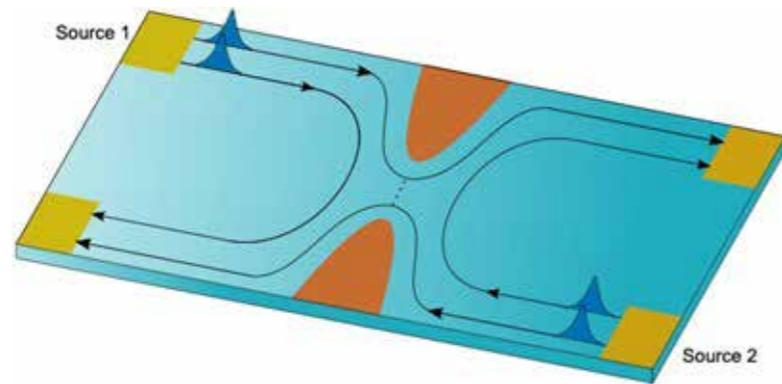
A quantum Hall interferometer. Electronic states are injected into the waveguides (edge channels) by the two sources and interfere at the central beamsplitter.
