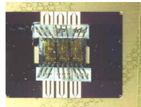
A complete all carbon-based electronics system using 3D CNT based via stacking, graphene enhanced inkjet printing as well as graphene devices.
