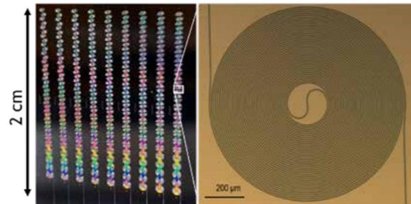
Photograph of a silicon-nitride spiral waveguide structure used to demonstrate the first CW optical parametric amplifier
