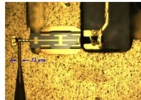
A 3.5-THz,  $\times 6$ -harmonic Schottky diode mixer published in *IEEE Transactions on Terahertz Science and Technology*, 2021.
