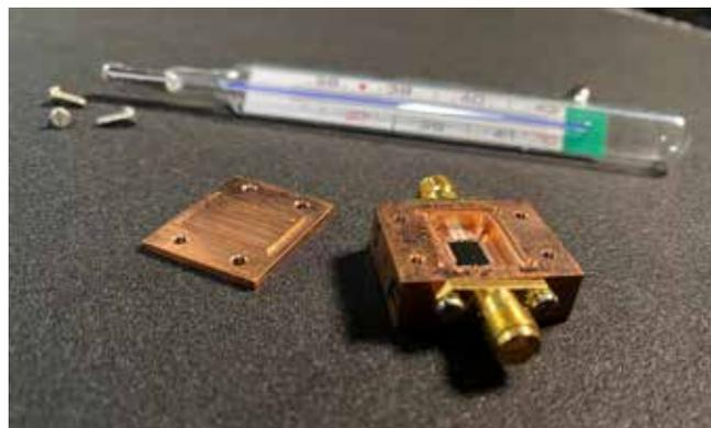
Researchers at Quantum Technology Laboratory, MC2 have developed a novel type of thermometer that can simply and quickly measure temperatures during quantum calculations with extremely high accuracy. The breakthrough provides a benchmarking tool for quantum computing of great value – and opens up for experiments in the exciting field of quantum thermodynamics.
