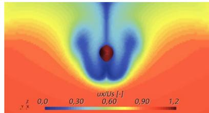
Flow into the propeller (wake)
