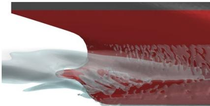
Coherent flow structures in the aft part of a hull
