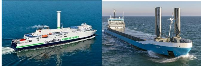
A ro-ro ship equipped with Flettner rotor (left) and a cargo ship equipped with two wings (right) with 1 year of performance monitoring data in this thesis project
