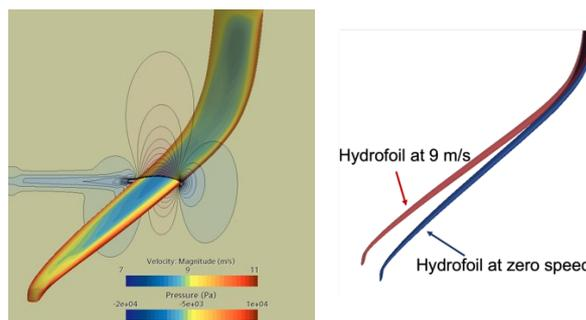
Figure 2: Hydrofoil subject to hydrodynamic loading and its ultimate deformation.
