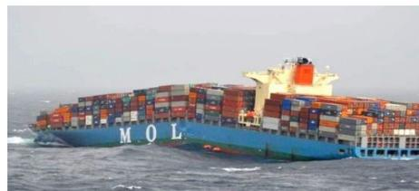
Fig 1. Ship structural damage caused by a severe wave loading.
