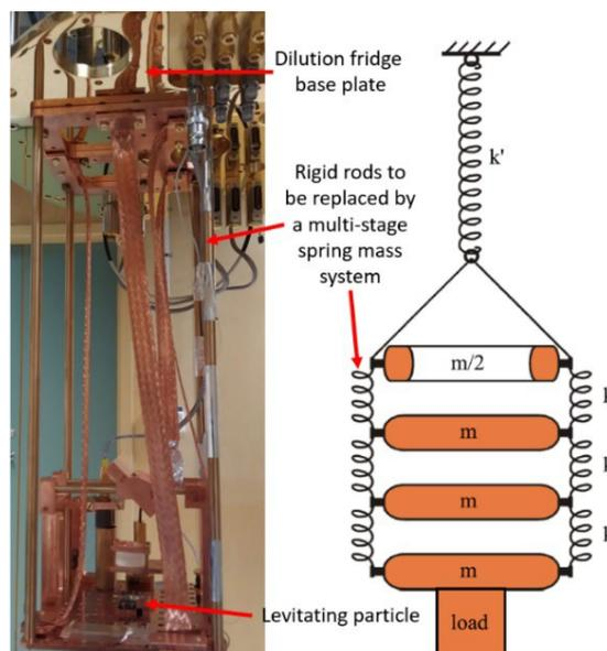
remain isolated from the environment for cooling its motion. However, various external factors influence the particle and cause heating. A dominant noise source comes from external mechanical vibrations originating from the pulse tube compressor of the dilution refrigerator, as well as surrounding noise from the building.
