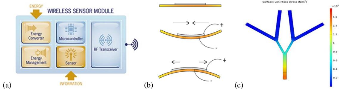
Figure 1: (a) Schematic of IoT sensor node based on energy harvesting; (b) Piezoelectric principle used for vibration-based energy harvester technology; (c) Finite Element simulation for stress distribution of a fractal-based harvester structure.
